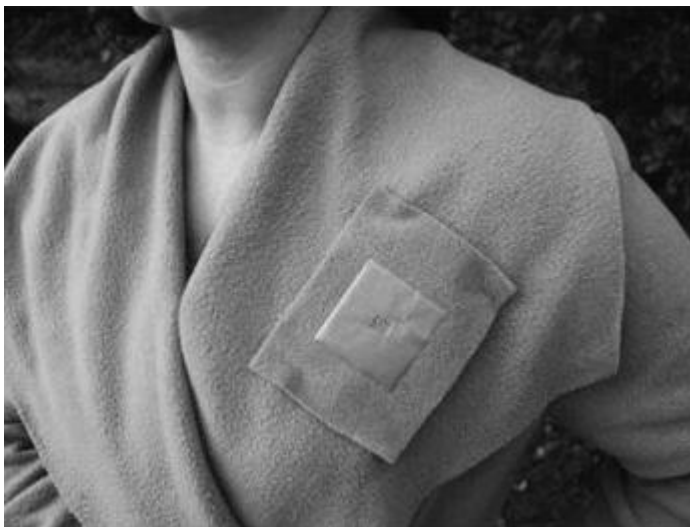
Fabric microstrip Antenna
